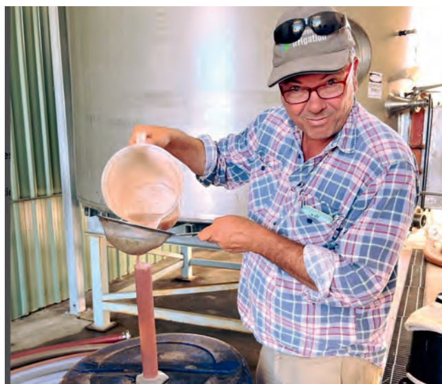
• Joch testing baumé levels of the Pinot Noir in preparation for harvest
